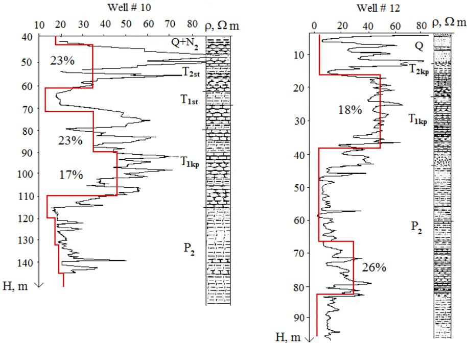
**Figure 4.** Borehole logs, resistivity as result of interpretation of time domain and porosity (in %) obtained using fractal model.
