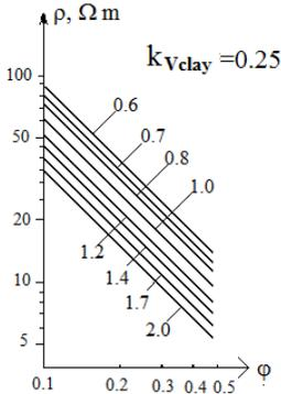
**Figure 3.** Calculated resistivity versus porosity coefficient of three component sediments. Index of curves is salinity of water (g/l). Volume of clay in unit is 0.25 (25%).
