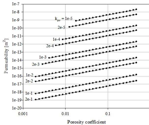
**Figure 2.** Permeability versus porosity for different amounts of absorbed water.
