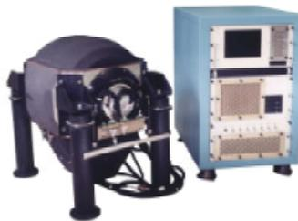
**Figure 2.** Gradiometer system: platform & electronics.
