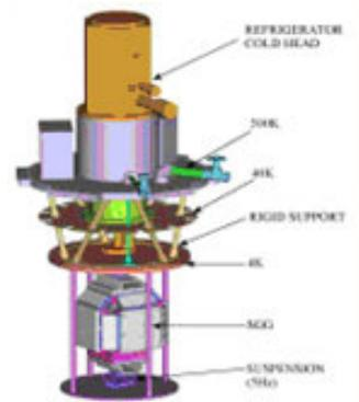
**Figure 7.** Layout of the Gedex HD-AGG<sup>TM</sup>.
