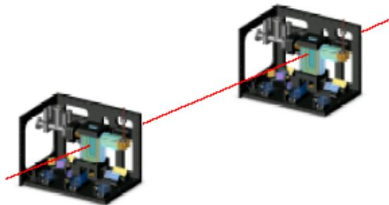
**Figure 5.** Dual AI accelerometer gradiometer concept.
