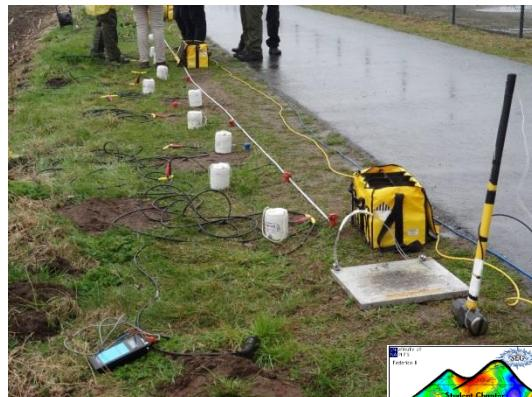
We used two different kind of geophones, the cable connected and wireless.
