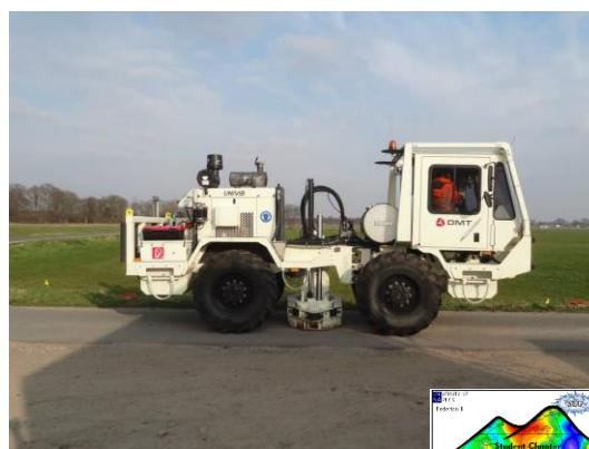
The energy generated from the Univib was recorded using a Sercel 428/208 acquisition system, also provided by DMT. The system comprises 240 recording channels, which record the summed
